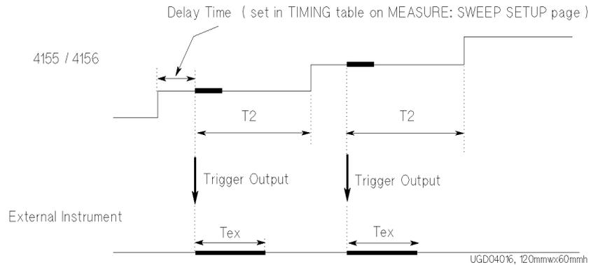
T2 : step delay time ( set in STEP DELAY field on MEASURE: OUTPUT SEQUENCE page )
