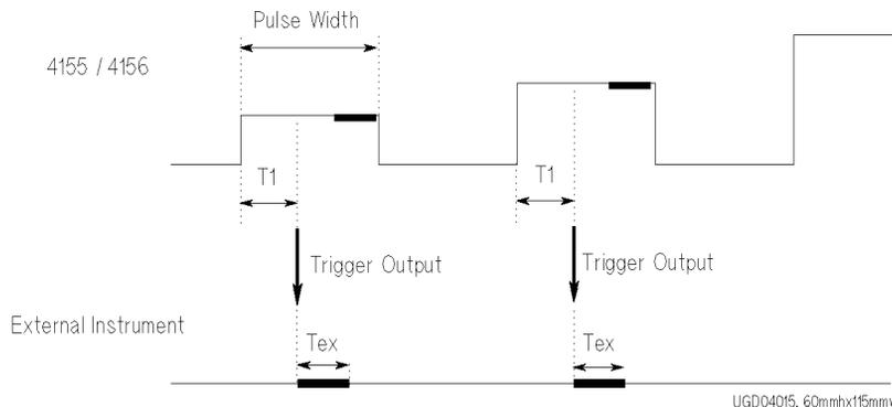
T1 : trigger output delay time
